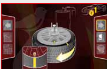
Match-Mounting procedure (rim-tyre)
