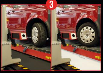
Steering - wheel parameters measurement
