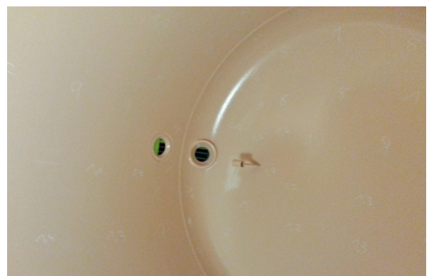
Coroflake lined vessel
