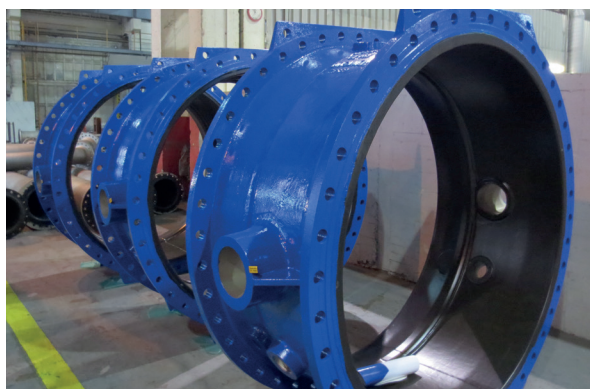
Rubber-lined flow-meter pipe
