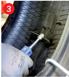
3 Clean the repair area using LIQUID BUFFER and a scraper.
