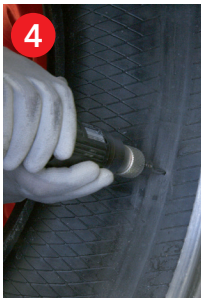
4 Prepare the puncture channel first from the tyre inside outwards, then from the outside to the inside.
