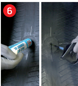
6 Apply CEMENT FD-BL on the buffed surface, fill the puncture channel with fresh cement and immediately insert the MINICOMBI plug.
