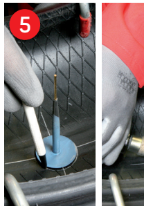
5 Buff the inner liner until you get a completely smooth surface (RMA-2) and clean the buffed area.
