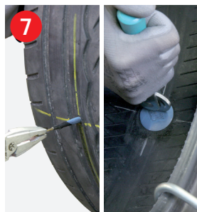
7 Pull the MINICOMBI plug outwards as far as possible and stitch the MINICOMBI base.
