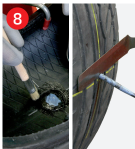
8 Seal the MINICOMBI base and any still exposed buffed areas with INNERLINER SEALER, reinflate mounted tyre and then cut the stem.
