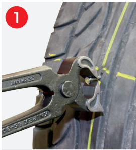
1 Locate and mark the damage. Take or screw out the foreign object.
